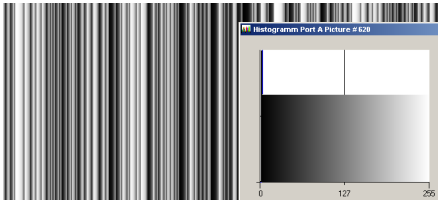
Figure 4.23: LFSR test pattern received at the frame grabber and typical histogram for error-free data transmission
