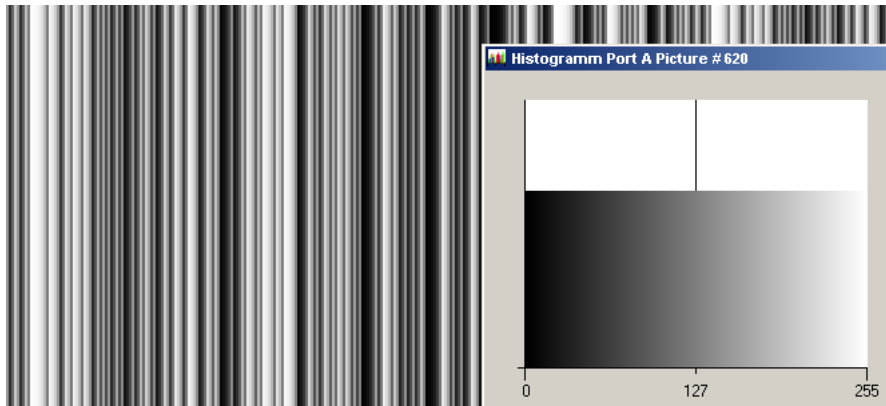
Figure 4.13: LFSR test pattern received at the frame grabber and typical histogram for error-free data transmission
